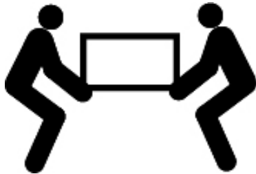
Figure 2-1. Lifting the centrifuge at both sides.
